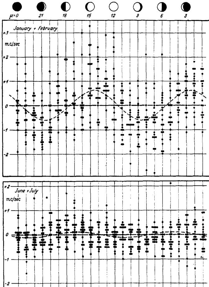
Fig. 14—Daily noon-values of  $fF_2$  at Huancayo, on undisturbed days, in deviations from 27-days averages, arranged according to the phase  $\mu$  of the mean moon, to show lunar tidal influence in the course of a lunar month.
