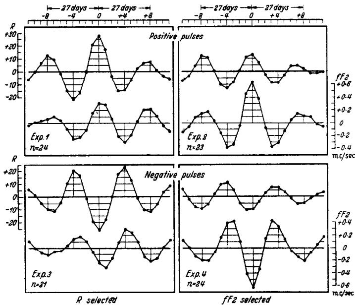
Fig. 8—Results of synchronization-experiments for sunspot-numbers  $R$  and critical frequencies  $fF_2$  at Huancayo.  $n$  = number of epochs superposed.
