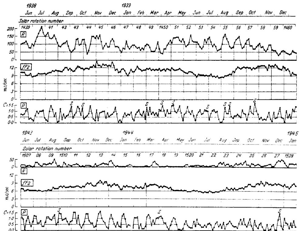
Figs. 3 and 4—Eighth-values (that is, eight values per solar rotation of 27 days) for sunspot-numbers  $R$ , noon-values of critical frequency  $fF_2$  at Huancayo, and solar particle-radiation  $P$ , for two intervals of 22 rotations each, near sunspot-maximum and near minimum.
